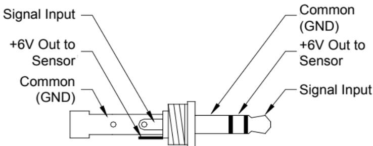
**Figure 2 Input Connector Detail (Stereo plug)**
