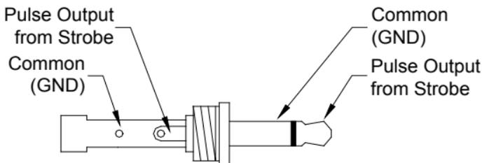
**Figure 3 Output Connector Detail (Mono plug)**
