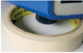
Placing the left side of the case on a roll of tape or other lift will prevent the speed knob from pushing the PCB out of the retaining slots when aligning all.
